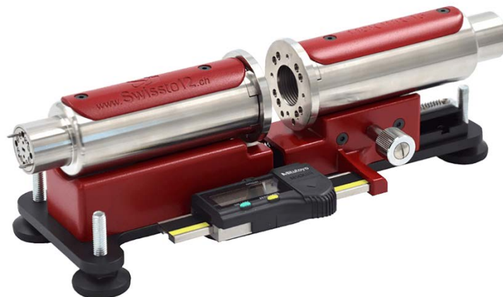
Fig.9.1: The material characterization kit (MCK) from SWISSto12 [P2] is a dielectric material characterization solution based on high-precision transmission/reflection mm-wave measurements under controlled and thus highly reproducible conditions. The acquired setups operate in the ranges from 26 GHz to 40 GHz (WR28, K a band) and 110 GHz to 170 GHz (WR6, D band), whereas the first setup addresses the 5G frequencies under investigation. The material probe is fitted into the gap between the two horn antennas.
