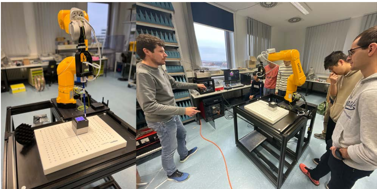
Fig.9.13: The DASY8 MP8B TX2-60L system [P3]: (left) front view of the robotized scanner setup; (right) typical scene during installation and corresponding instructions by the SPEAG personnel also showing the controller unit in the background.
