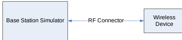
Figure 9-4 Power Measurement Setup – NR FDD
